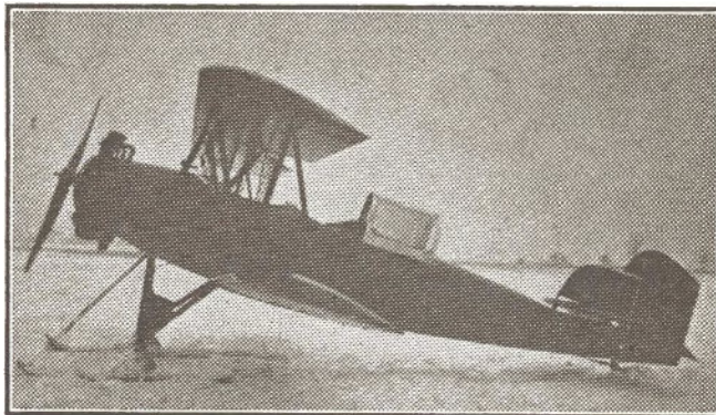
Another fellow who went in for a sliding hatch was the owner of this Consolidated Fleet. And he very much needed such protection for his wintry flying, which, as you see, also called for skis. The hatch slides all the way up under the wing, there. Yes, it does look a bit strange on this job—but it keeps the weather out.
